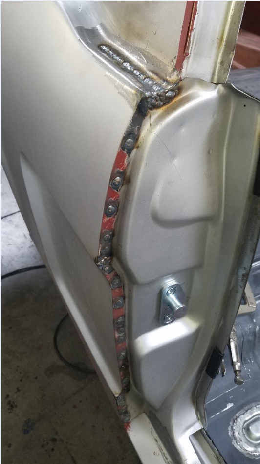
The quarter panel was plug welded in the door jamb.
