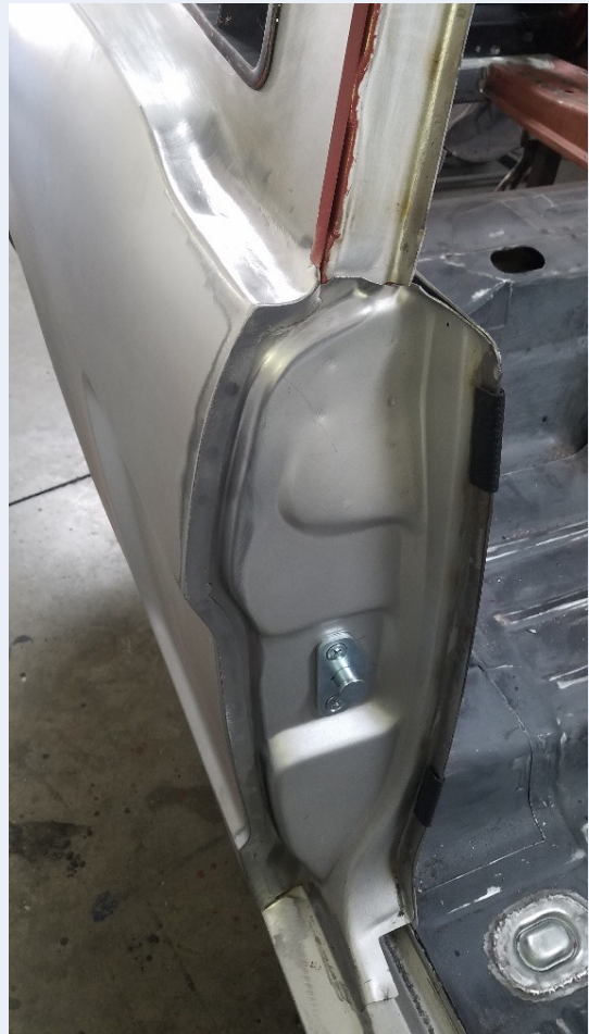
After grinding the welds it looks like it was never done.
